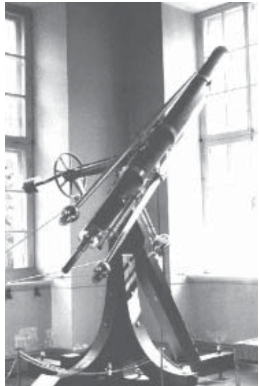
The 9-inch Fraunhofer refractor at Dorpat, used by Wilhelm Struve for his study of double stars.
