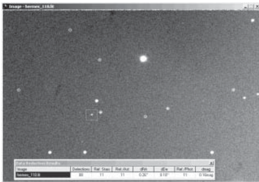
Figure 1. A screenshot showing an image of asteroid 1937UB (Hermes) being reduced using Astrometrica . The circled stars have been identified and correlated with stars in the USNO-A2.0 catalogue. A total of 11 stars are used in the reduction and these have RMS position errors of 0".26 in RA and 0".18 in Dec. Hermes is the object in the box.
