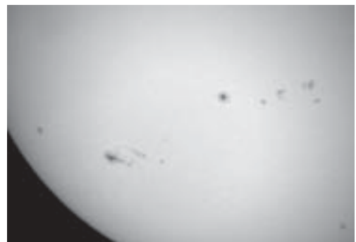
Figure 7. Sunspots, 2002 September 22, 80mm refractor with Baader AstroSolar Safety Film (visual) filter. Imaged with Nikon Coolpix 900 digital camera coupled to 26mm Plössl eyepiece using ScopeTronix adapter. Self-timer and auto-exposure used.
