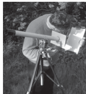
Viewing the Sun by the projection method. (Neil Bone)
