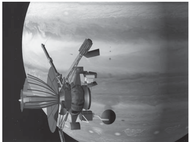
Artist's impression of the Galileo probe in orbit around Jupiter, with its main antenna only partly deployed. NASA
